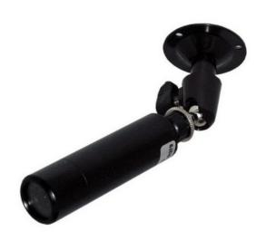
This camera includes an **On-Screen Display** (OSD) accessed using the in-line OSD joystick, which allows one to configure the camera's advanced settings to compensate for specific environmental factors and light levels. The OSD joystick also allows the user to easily toggle between the AHD, HDCVI, HD-TVI, and 960H video formats.
